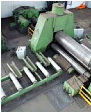
▲ Bending roll machine – 2,200 ton capacity.
