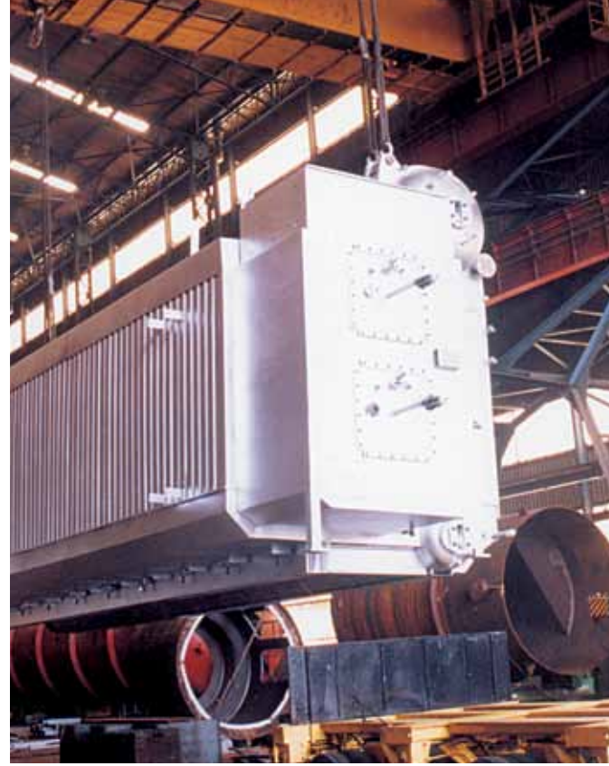
▲ Compact FM boiler – 80 ton/hour.
