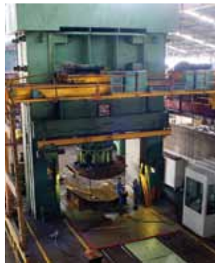
▲ Hydraulic press with 6,000 ton capacity (4.5m in height, 5m in width).
